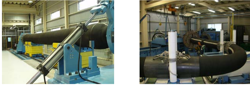
Figure 1: Prototype testing dynamic torsion and bending status (formal certification test)
