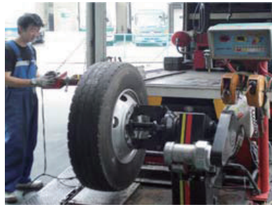
Replacement, removal, air adjustment work of tires using a machine for tire replacement work for trucks and buses.
