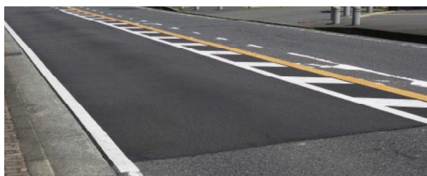
Section of public road surfaced with the new material for tests (the part of the darker color)
