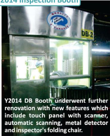
Y2014 DB Booth underwent further renovation with new features which include touch panel with scanner, automatic scanning, metal detector and inspector's folding chair.
